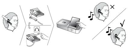
Figure 11: Setting the clear dial-tone switch manually
